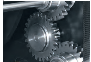
Precise gearing provides even line take-up and release.
