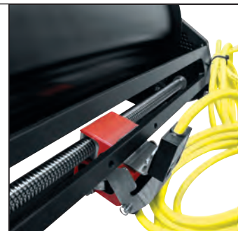
The screw design positions the screw close to the drum, reducing winch size.
