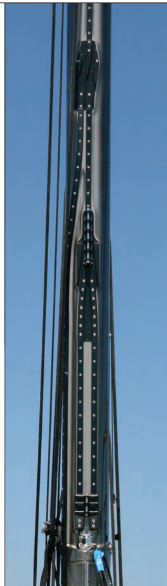
The Trysail Switch system integrates with the Switch T-Track Battcar system by sharing a single mast track to reduce weight aloft.
