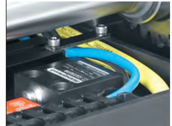
Two inner magnetic switches factory-set at the feeder's stroke limits prevent overtravel. Two outer fail-safe limit switches automatically engage the brake.
