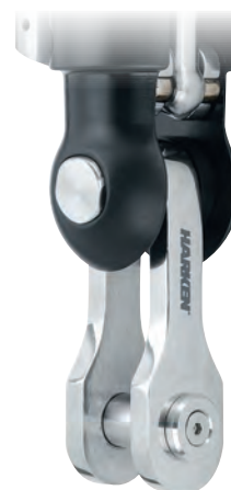
Harken recommends attaching a toggle to the cylinder's bottom clevis to accommodate stay movement. Standard eye-jaw toggles fit all Harken cylinders.
