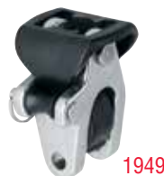
Toggles have a low pivot point to handle mainsheet loads up to 40 degrees from vertical, while allowing cars to roll freely.
