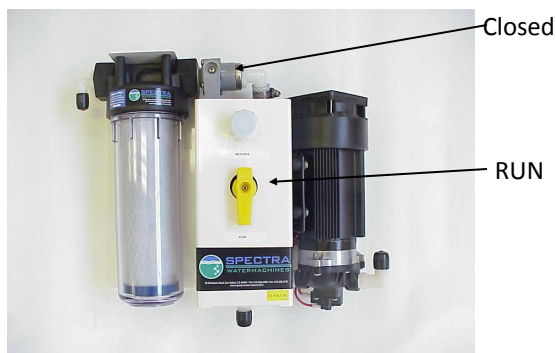
Feed Pump Module A with valves in the RUN Position:
