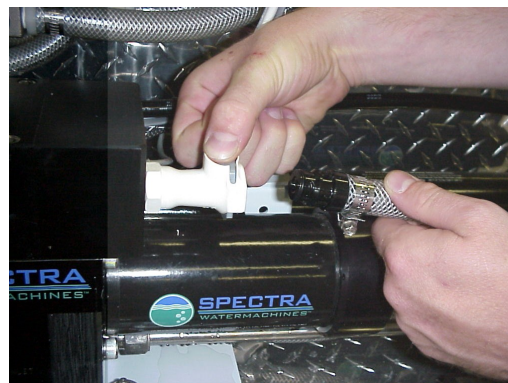
Connecting brine discharge hose:
