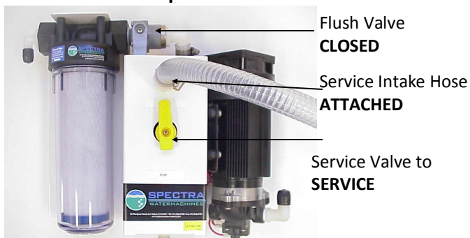
Valves in service position:
