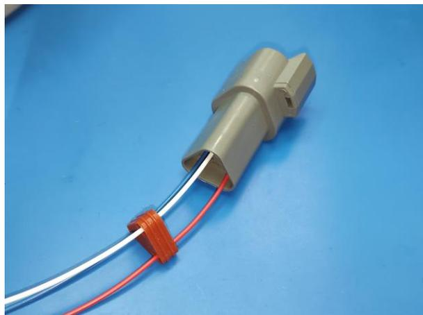
**Step 5:** Install water grommet on back side of connector.
